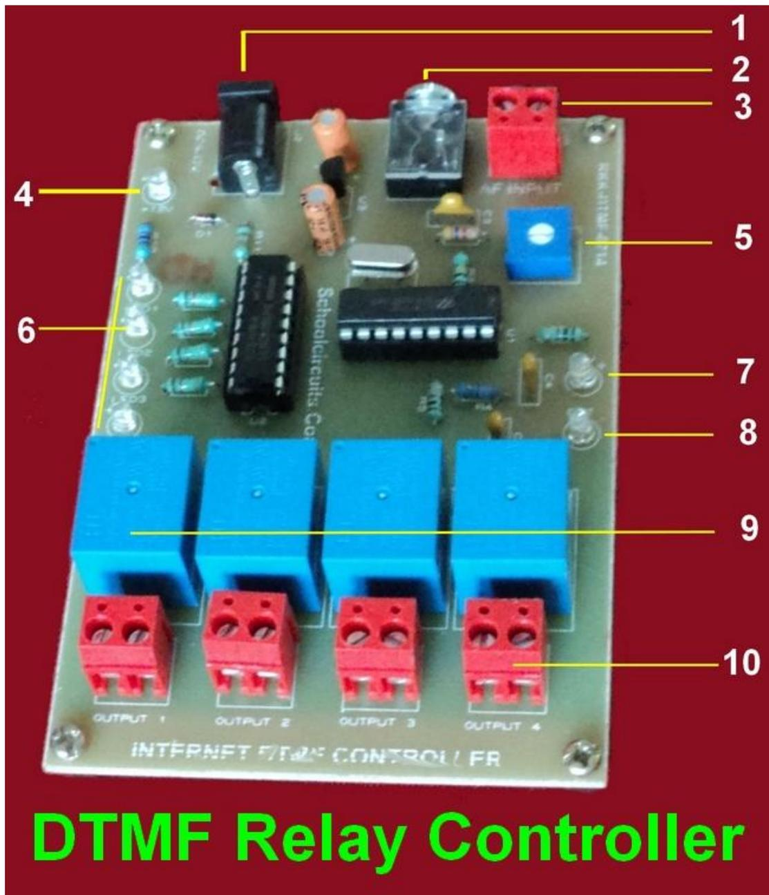
This high quality board is designed to get DTMF input from Internet / Mobile / Wireless receivers/ Computer for operation of 4 relays. AC 250 V AC rated Relays can control 4 devices attached to 4 outputs.
